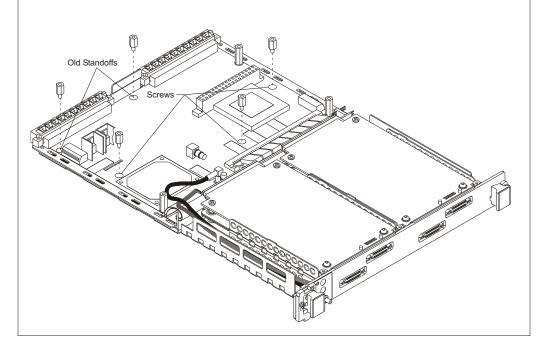
6 Using a T-10 Torx driver and the three screws saved from **Step 5**, attach the E1432-66541 assembly to the module.
