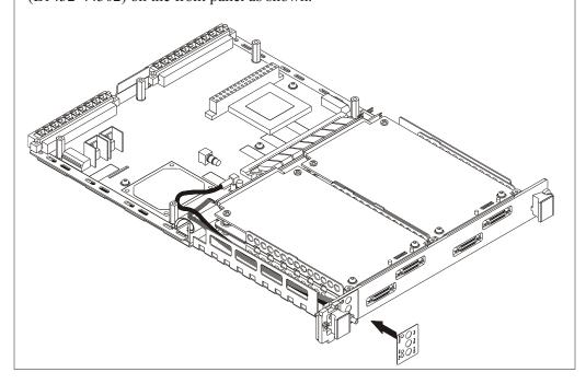
5 Using a 1/4 inch nut driver and a T-10 Torx driver, remove the three screws and the two standoffs and replace them with the five new standoffs (0380-4041) as shown in illustration below. **Save Screws.**
