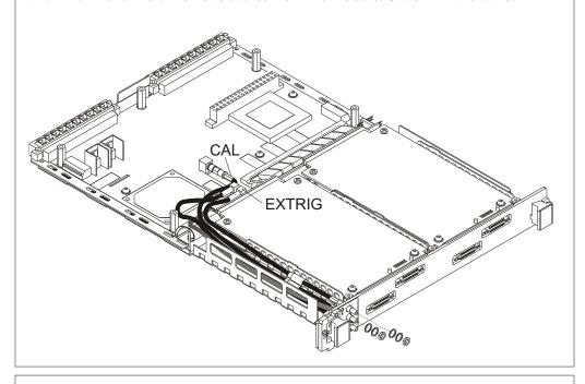
4 Remove the old label. Remove the tape backing and place the new label (E1432-44302) on the front panel as shown.
